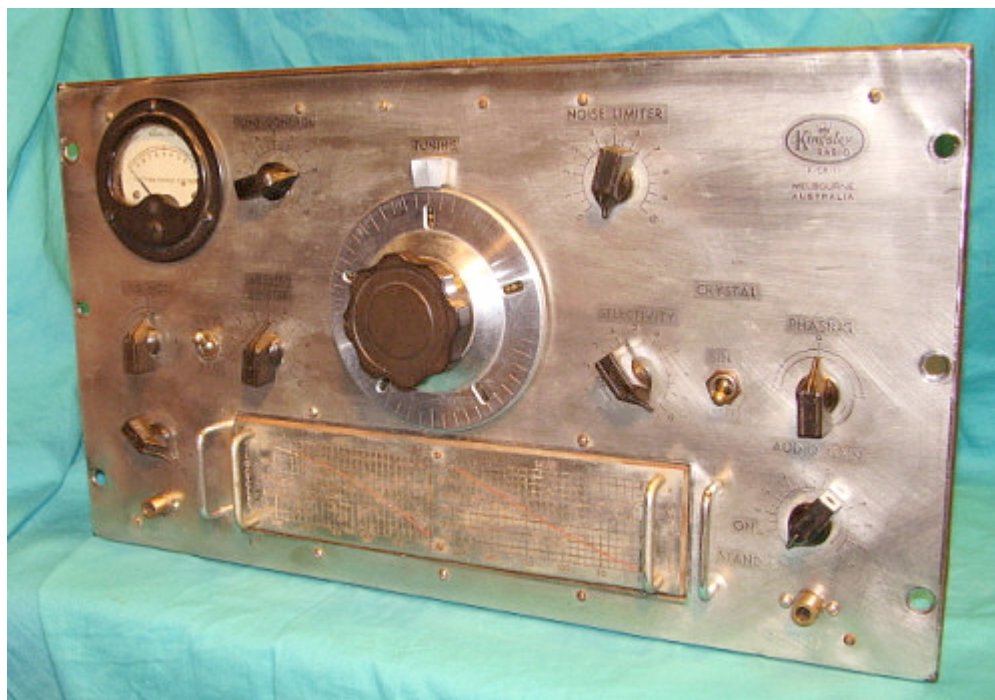
Fig.37: Kingsley HF Radio Receiver, Type AR7.
