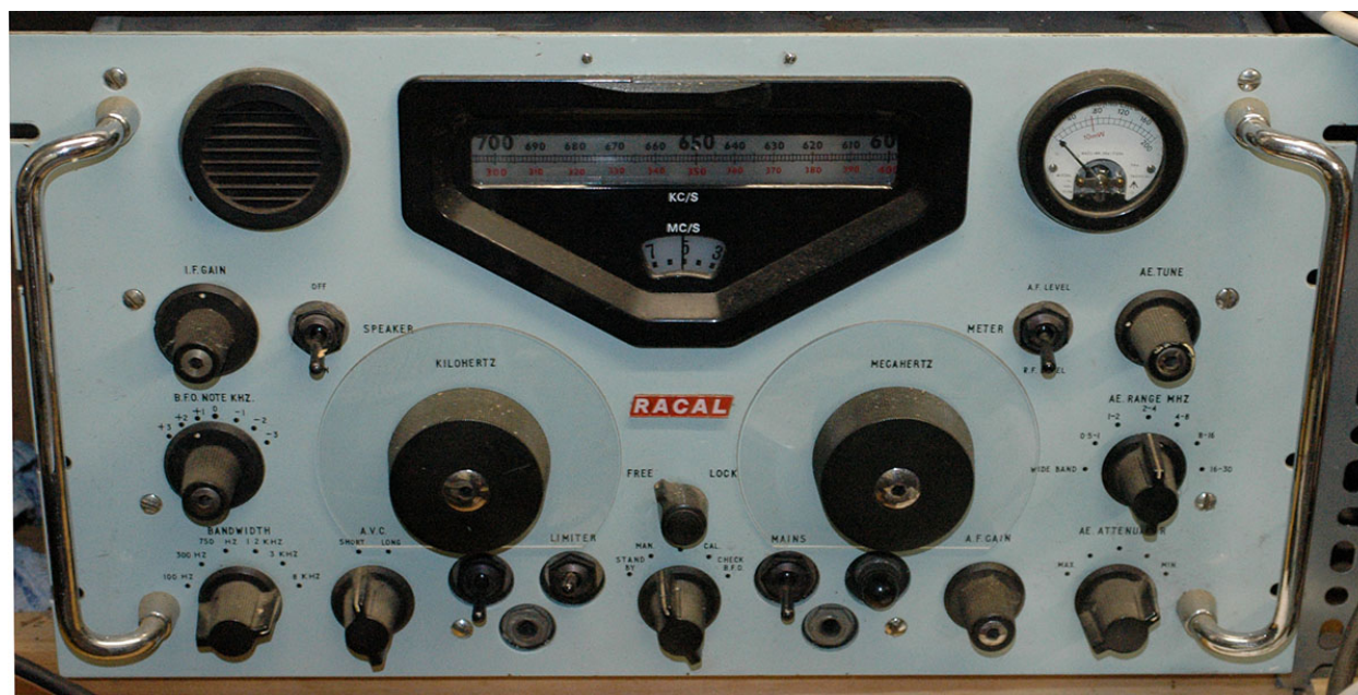
Fig. 34: Racal HF Radio Receiver, Type RA17.
