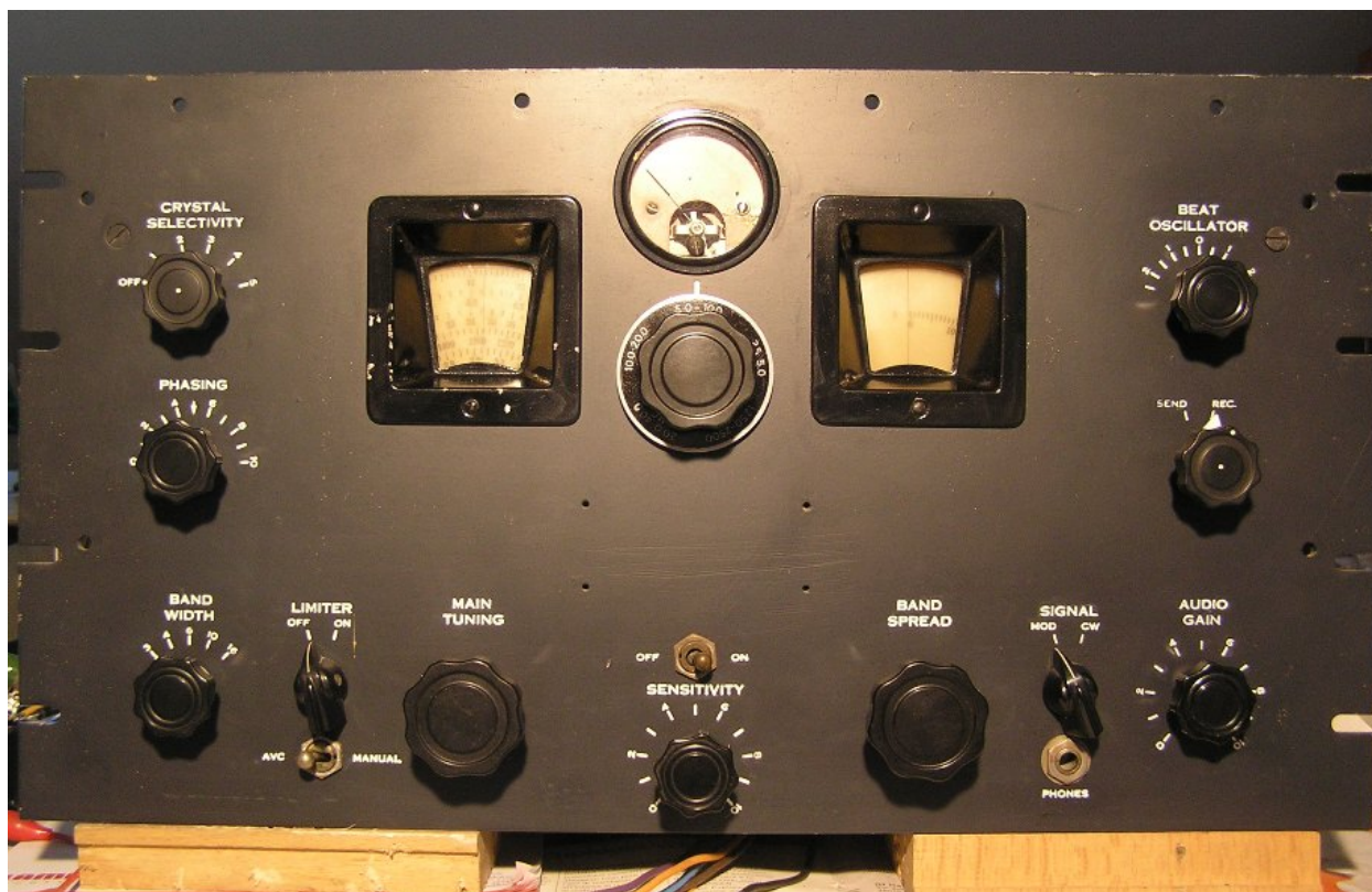
Fig. 32: Hammarlund HF Super-Pro Radio Receiver, Type BC-779-A.
