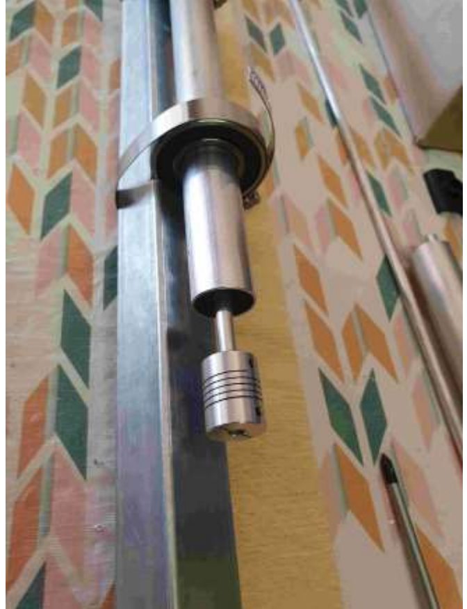
Flexible Shaft Coupler
