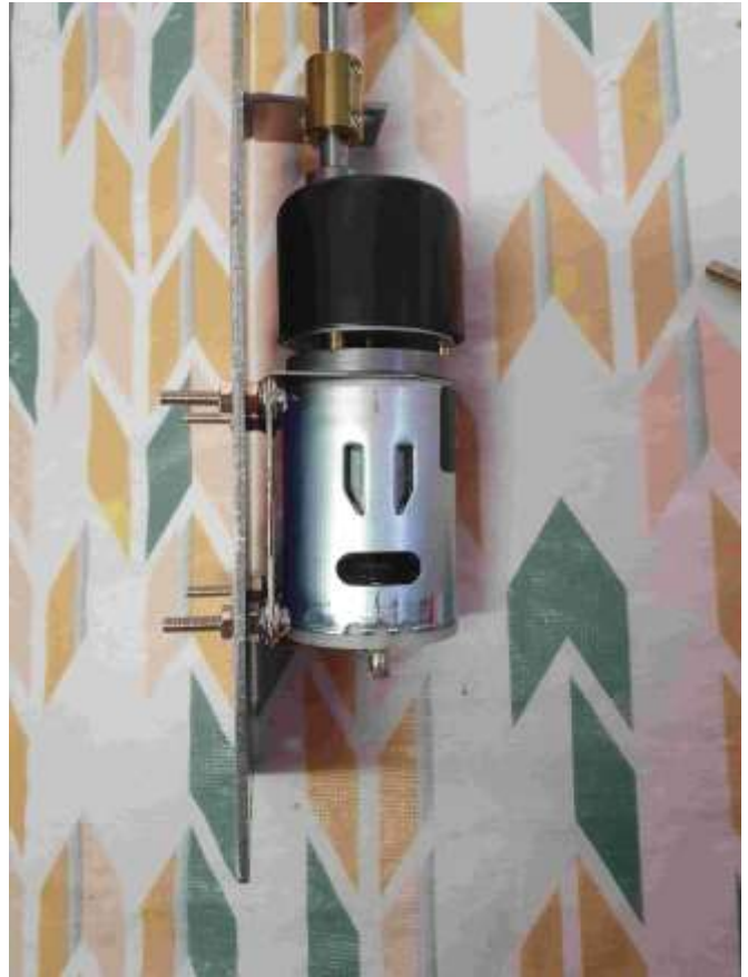
Flexible Shaft Coupler
